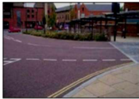
Photograph C.1,1 - Pigmented Hot Rolled Asphalt (Black binder + red coated chippings)
