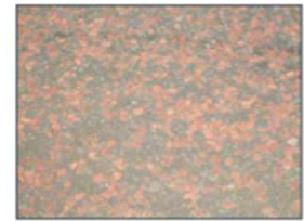
Photograph C.1,2 - Pigmented Hot Rolled Asphalt (Black binder + red coated chippings)
