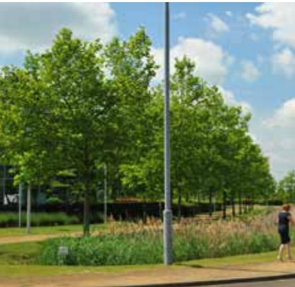
Planted attenuation basin
