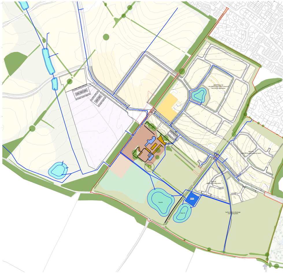
Illustrative location for attenuation basins
